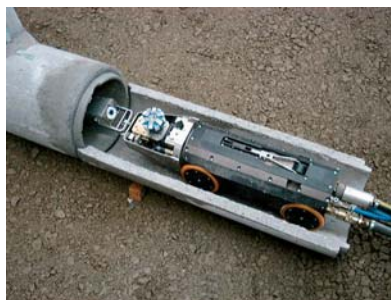
Milling robot with a pan and tilt camera
